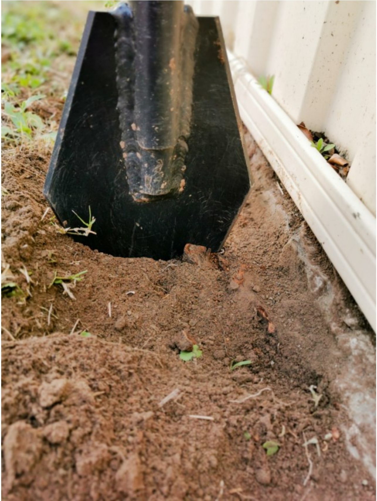
Slicing through more roots, the blade does not move from the cut, unlike a digging bar, which strikes all over the place, and can dangerously deflect off hard, slippery live roots.
