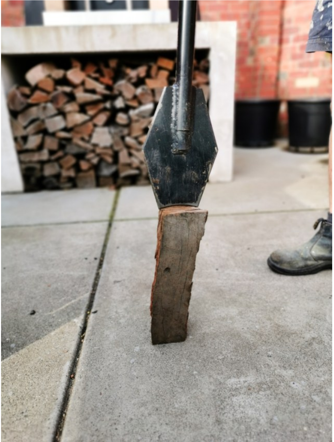
The crescent-shaped blade of the Slammer Tool blade sits securely on fairly narrow pieces of firewood timber.
