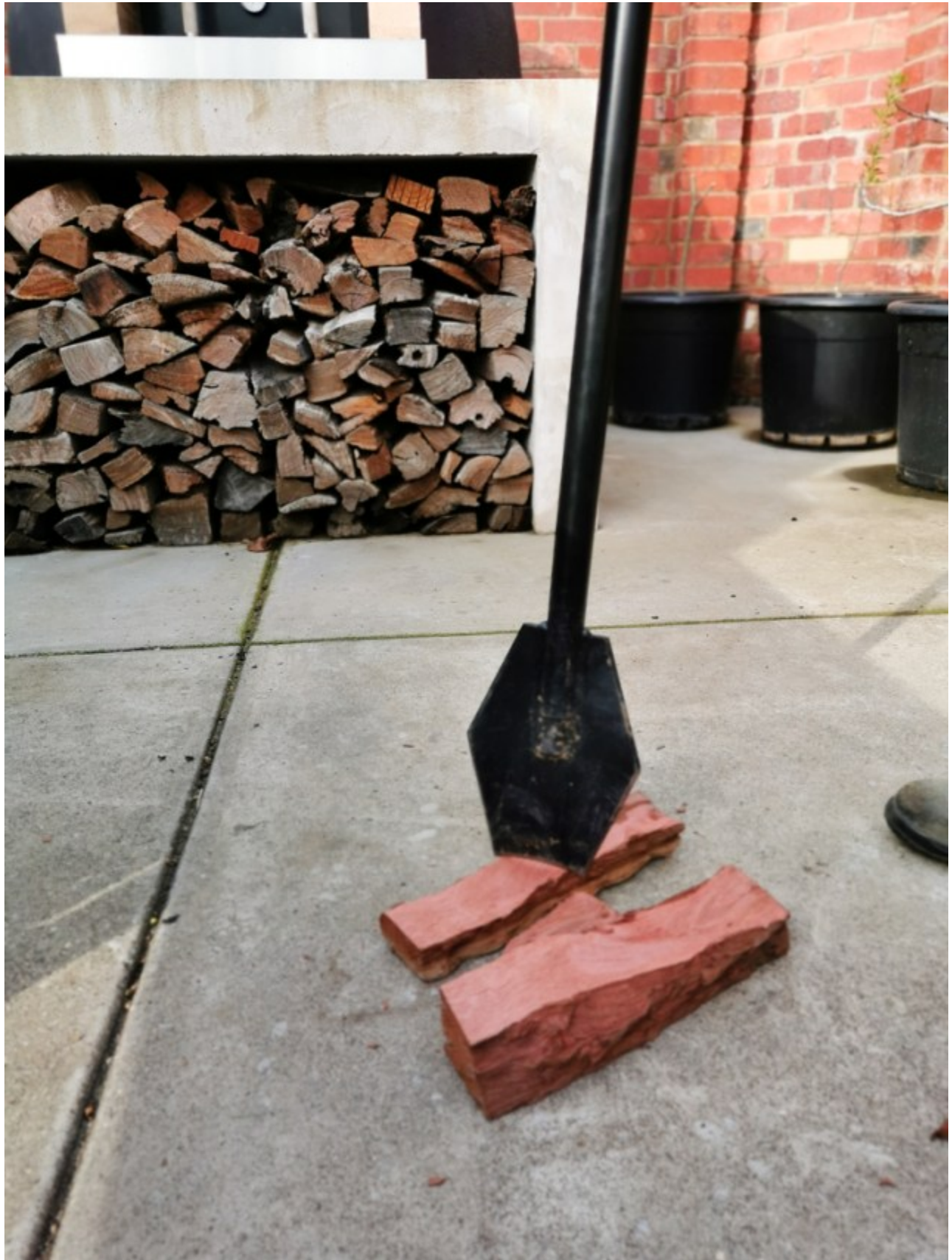
Redgum firewood easily split in two, the uneven split shows how bad the grain is in this dense wood, which plays havoc with axes and block splitters, and can easily cause deflection.
