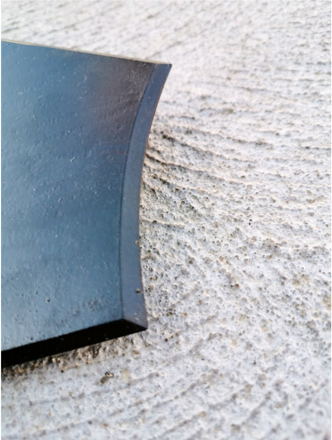
Close-up view of the Slammer Tool blade cutting edge
