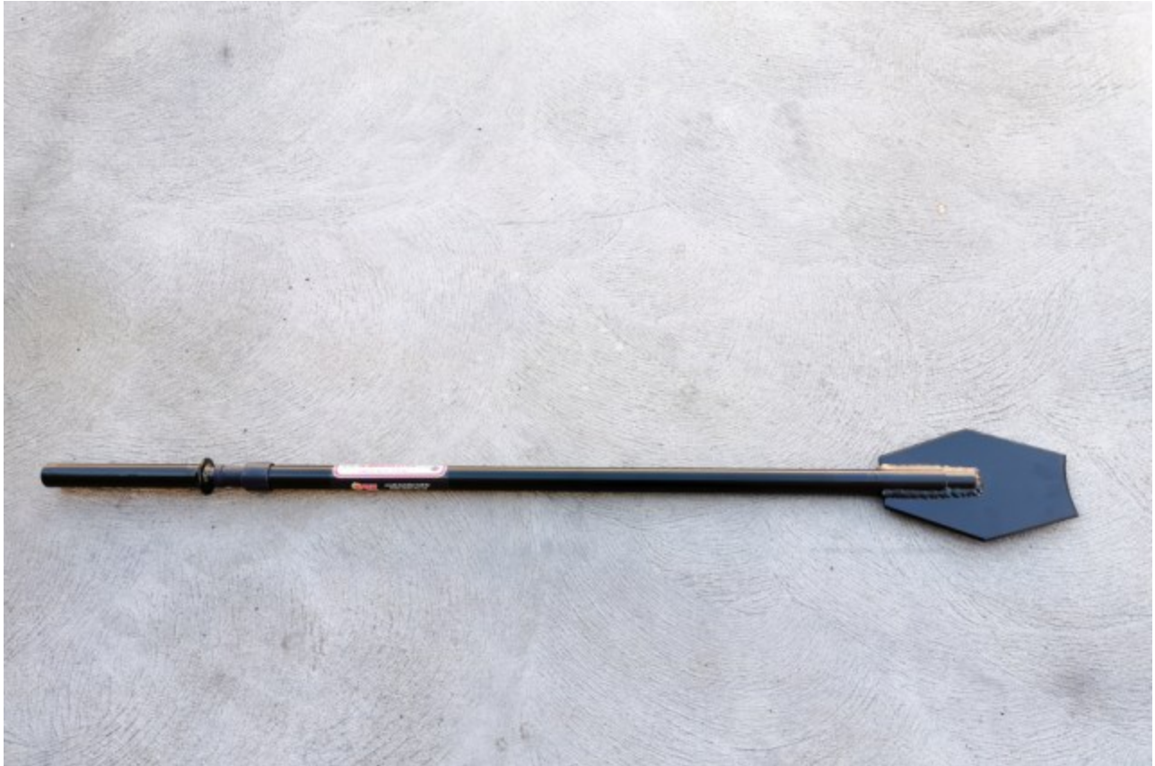
Slammer Tool assembled is 139cm (54") in length
