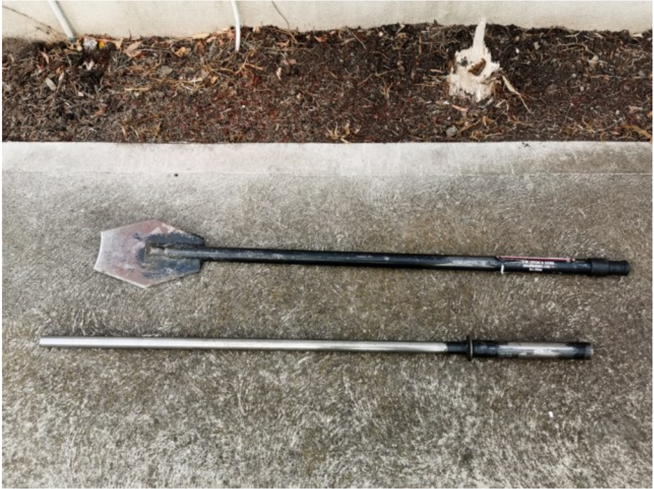
Slammer Tool separated into its two parts
