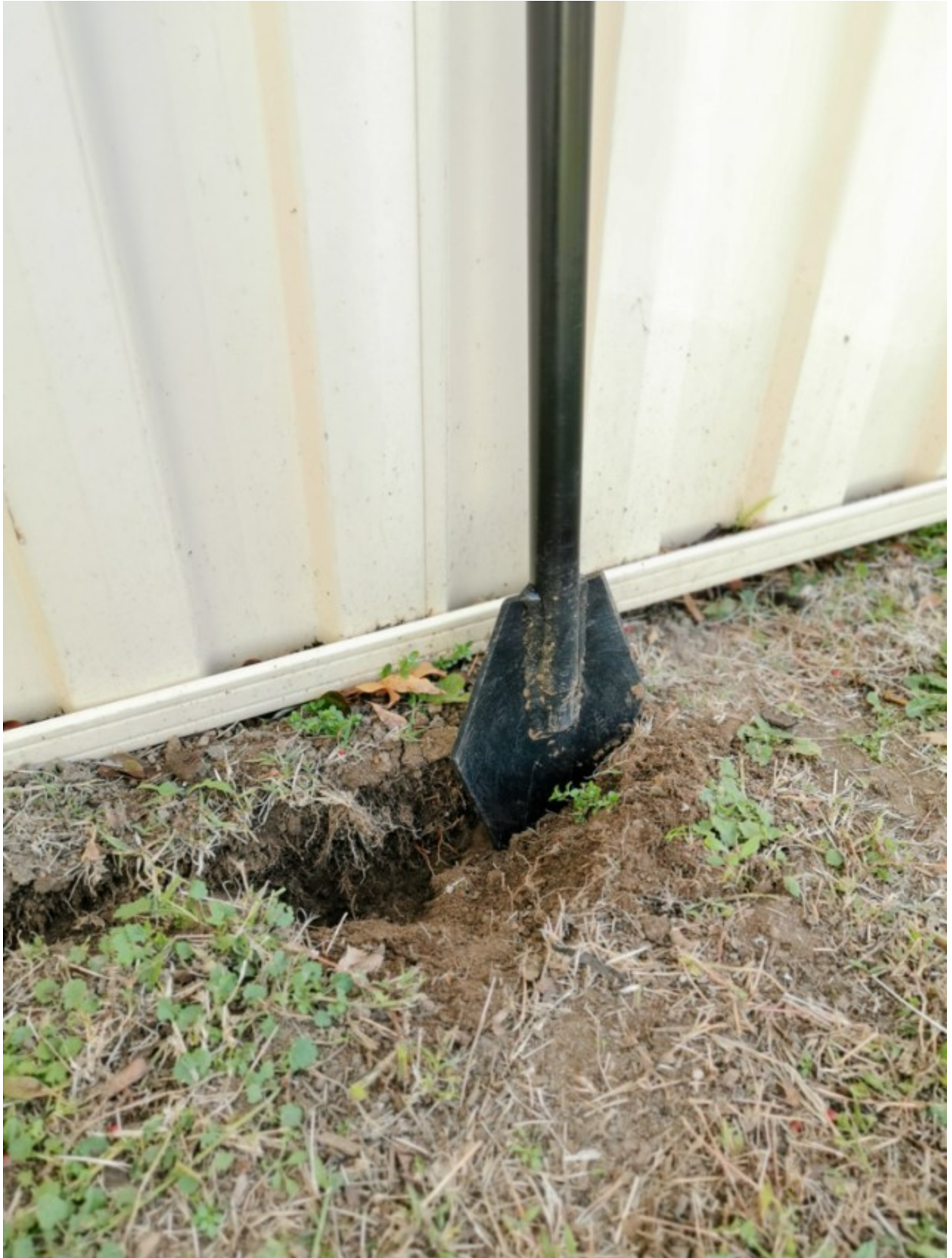
Cutting through compacted and root-filled soil is much easier with a Slammer Tool because the impact force goes into exactly the same place each time, every time, it's much more efficient.
