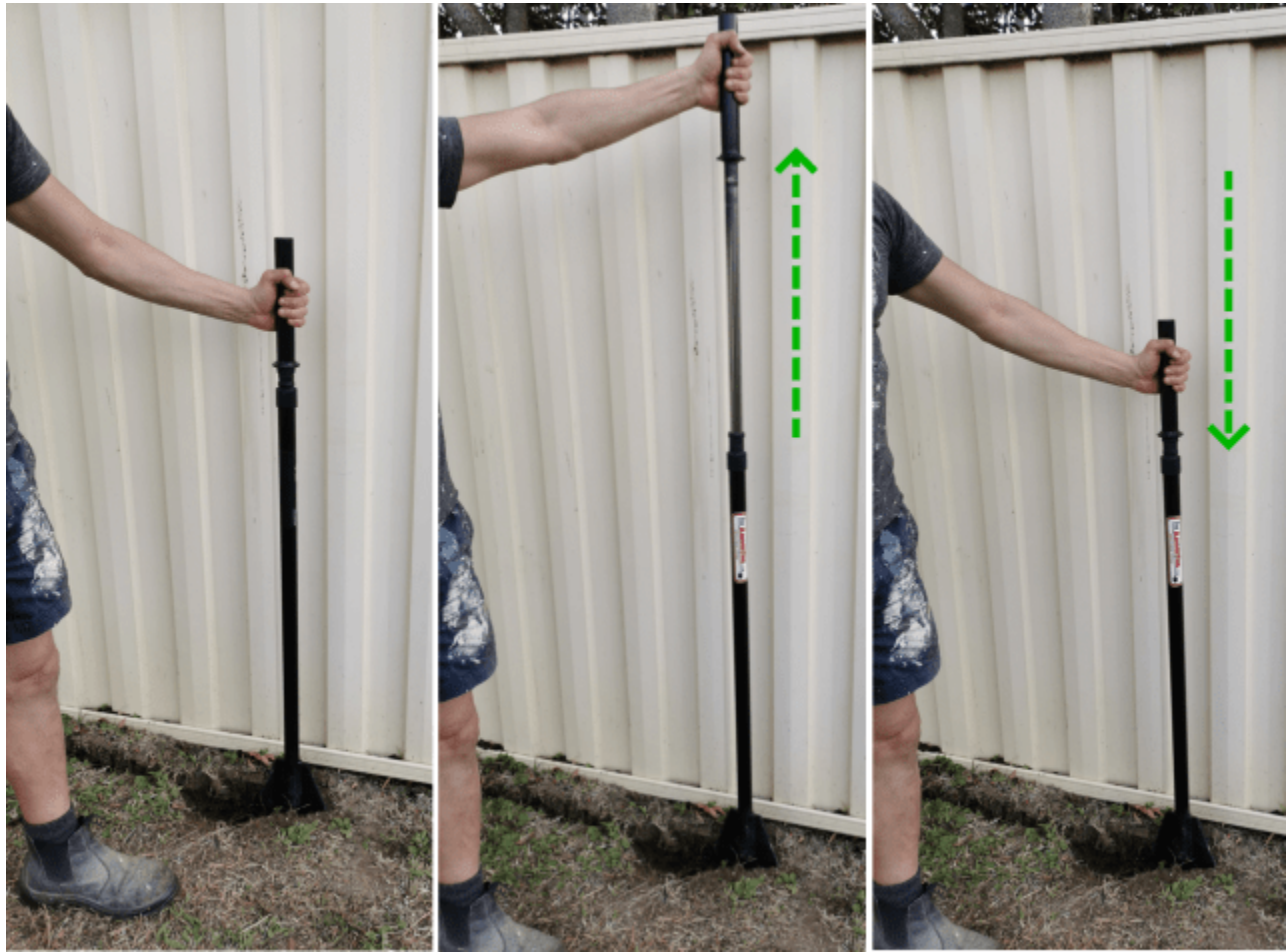
Three step operation – 1. place blade where cut is to be, 2. lift handle up, 3. slam it down hard!
