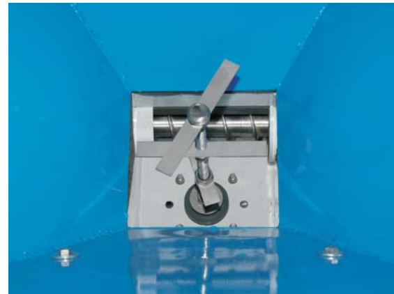
Mechanical stirrer at bottom of hopper
