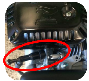
Disconnected spark plug
