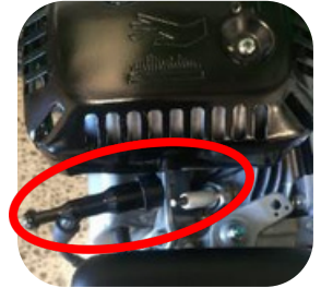
Disconnected spark plug
