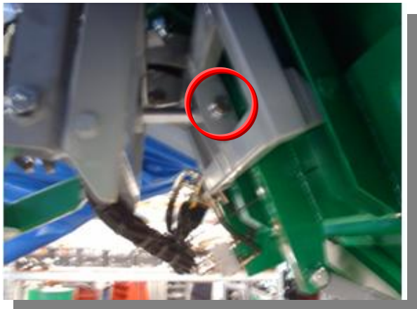
Picture 39: fastener piston – attachment orientation
