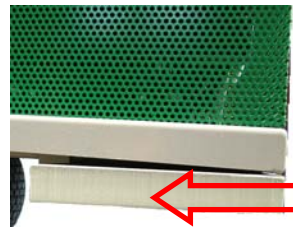
Direction to extract the ballast with the hydraulic floor jack
